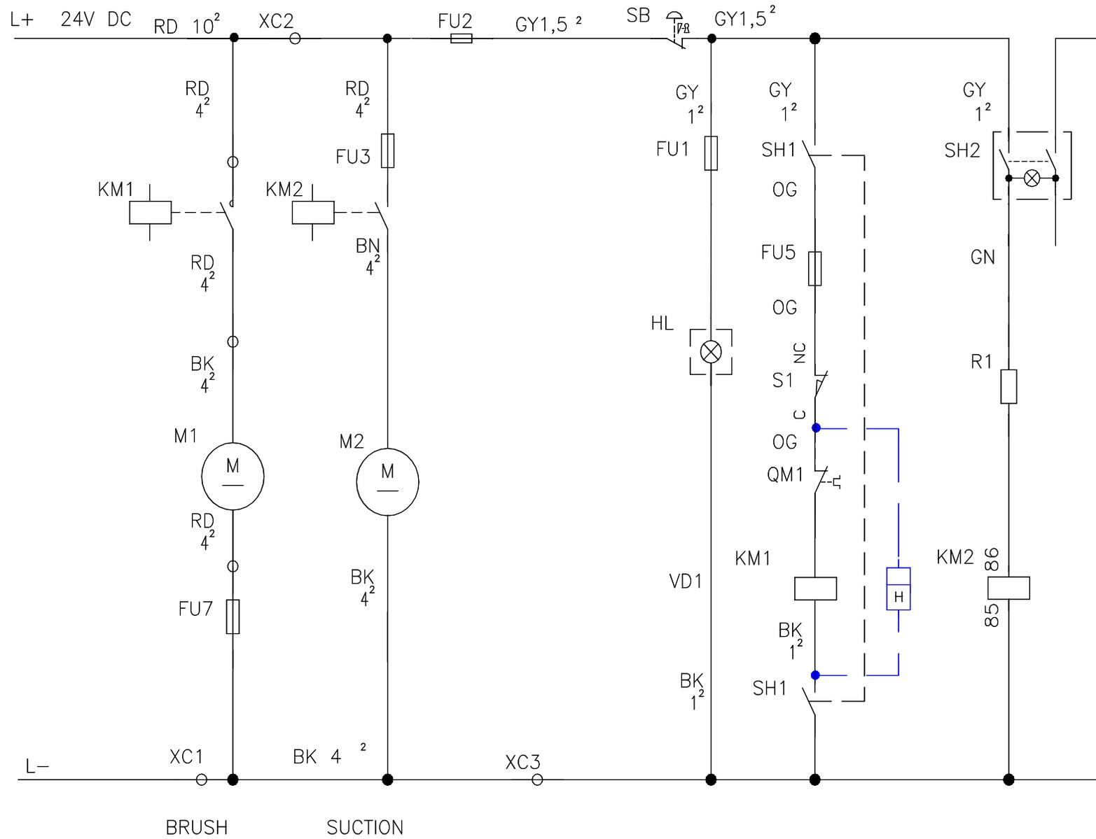
DESCRIPTION: ELEC. SCHEMATIC DIAGRAM / SCHÉMA ÉLECTRIQUE
