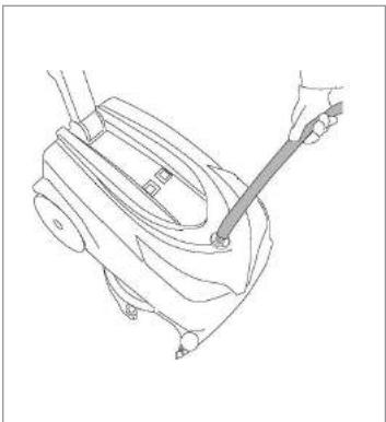
Fill solution tank with water and detergent.
