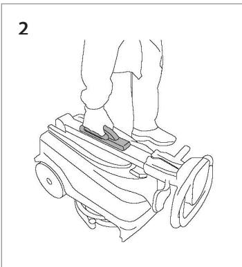
Lift the machine out of the box by the handle and set it down.
