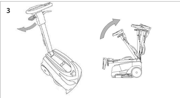
Pull the handle up at right angles to the machine.
