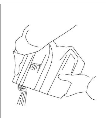
Remove the recovery tank from the machine to empty.
