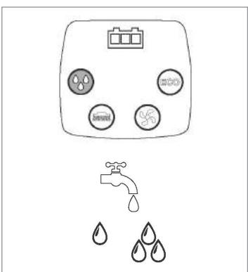
Press the solution button to set desired water level.
