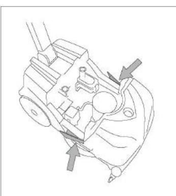
Press side latches to remove and empty the solution tank.
