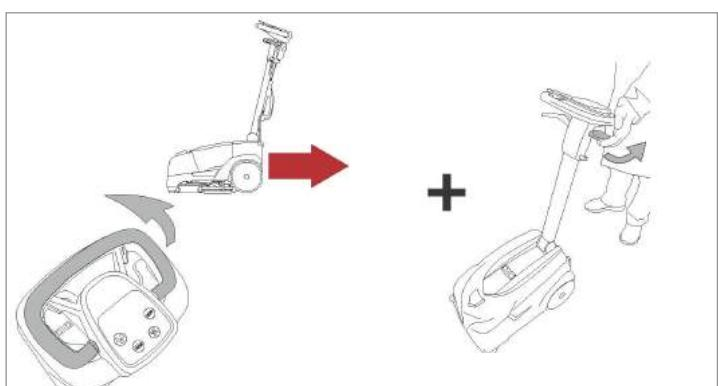
To clean in reverse, activate the front squeegee by pulling the front squeegee lever at the same time as the activation lever.
